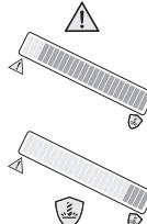
**WARNING!** If the beam of the overload indicator lights up close to the left symbol, the workload is very high. Reduce the workload or switch the motor off, otherwise the overload protection will be activated and the motor will be shut off automatically.
